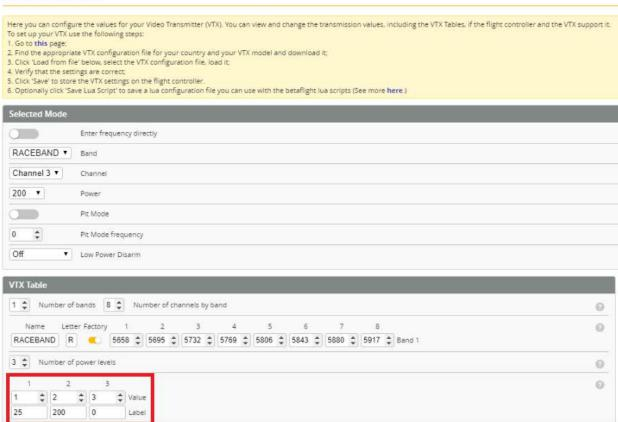
3 different RF power levels are specified on the above table. #1 and #2 specify 25 mW and 200mW RF power respectively, and #3 is to turn off RF output completely.
