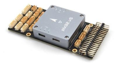
HolyBro Pix32 v5 is a new flight controller we have developed on the base of FMUv5 scheme, which can be regarded as a variant version of 'Pixhawk4'.
