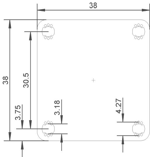
The ESC comes with a 30,5x30,5mm mounting hole layout designed for M3 and M4 screws.
