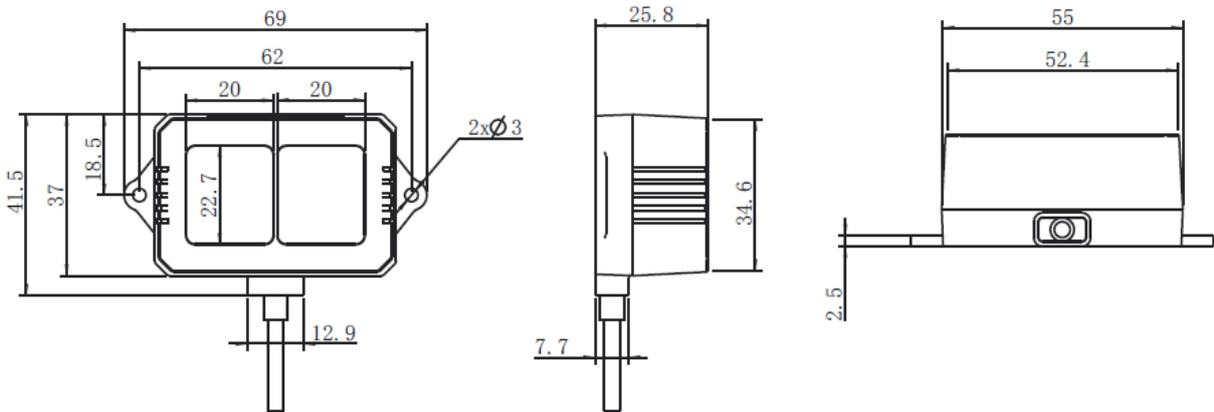
Figure 1: Constructional Drawing of TF02-Pro (unit: mm)
